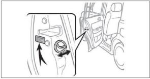
Move the lever to "LOCK," allowing the door to be opened only from the outside.
